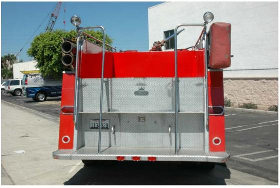
In order to spiff up the inside Oak planks were attached to the seats. A chrome strip was placed on the top of the rear diamond plate also the back diamond plate was primed and repainted.
