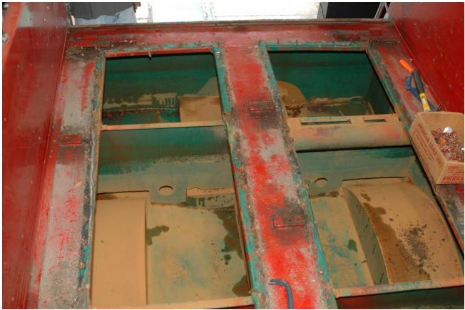
By removing these plates we can assure ourselves that all the water is out and it will also give us an area to feed our chains thru when we go to lift it out. Next it's time to disconnect the fittings that hook up to the pump and also we remove the bolts that hold the tank onto the frame.
