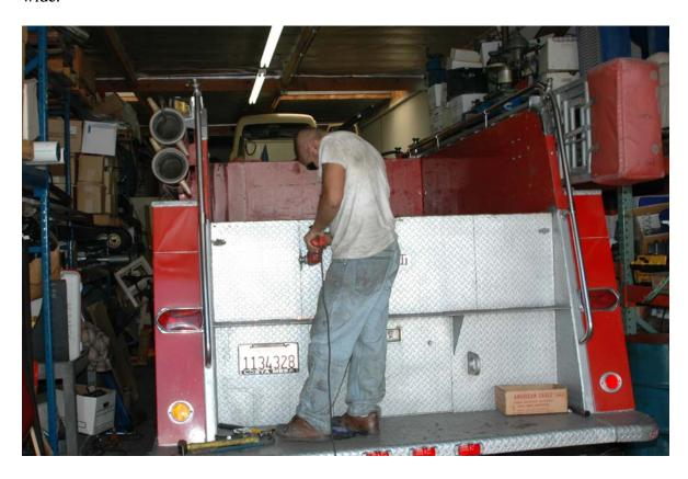
We use an abrasive cutoff saw and cut along the lines that we had laid out.
