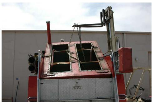
With all that done it's time to lift the tank out. We wrap a chain thru the openings and attach them to the forklift. We lift the tank straight out and set it to the side. In order for people and the casket to get in the back we need to cut the rear diamond plate. We call around and get the dimension of a casket. It turns out that they are 28 inches by 82 inches. With this information we decide to make the door opening 34 inches wide.
